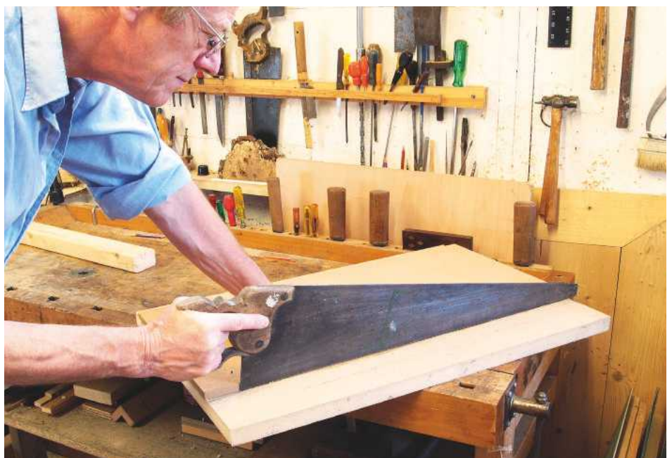
▲ Pic.10 Use a saw to make a slight dust groove at the junction between the two boards
